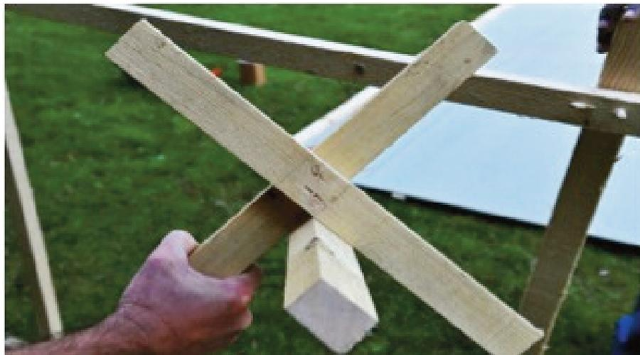
*Note:* This picture represents the prototype of the structural articulation built by Frank.
